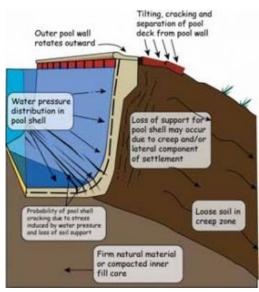
"[Slope creep] is where some of the hill is slowly moving with the pool... With that moving of the hillside, the pool is tilting or moving or losing support and it is causing a crack."
